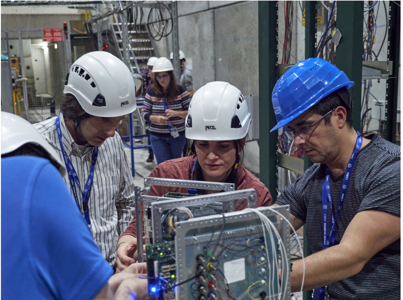
A team of experts preparing the experimental setup for testing the space-worthiness of the Intel Myriad2 system-on-chip for space applications.
