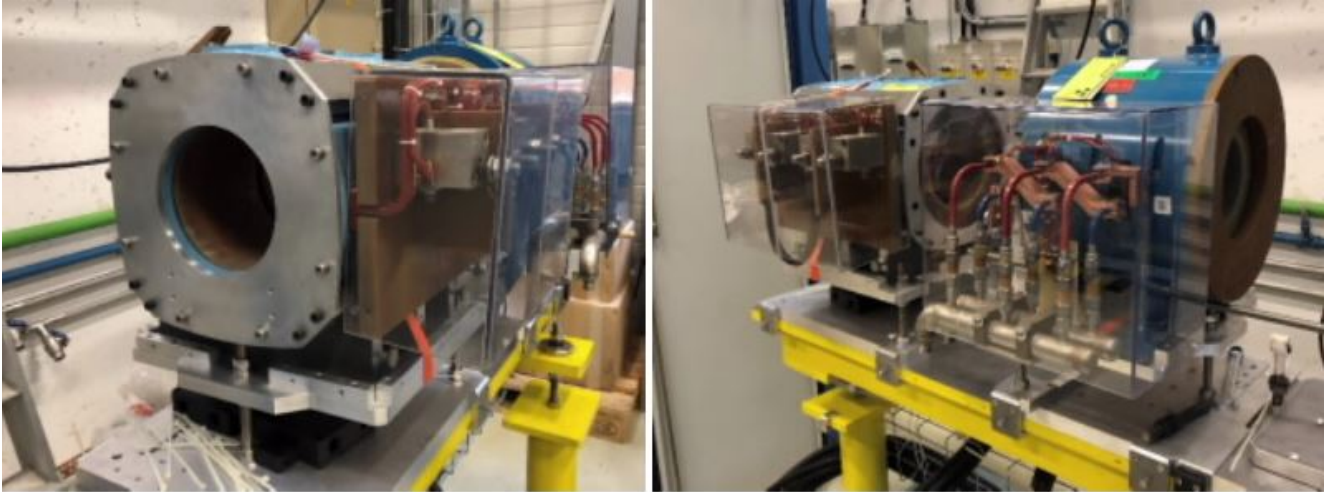
Figure 4. Electron Test Stand gun and collector magnet as from today's installation. (Image: CERN)
