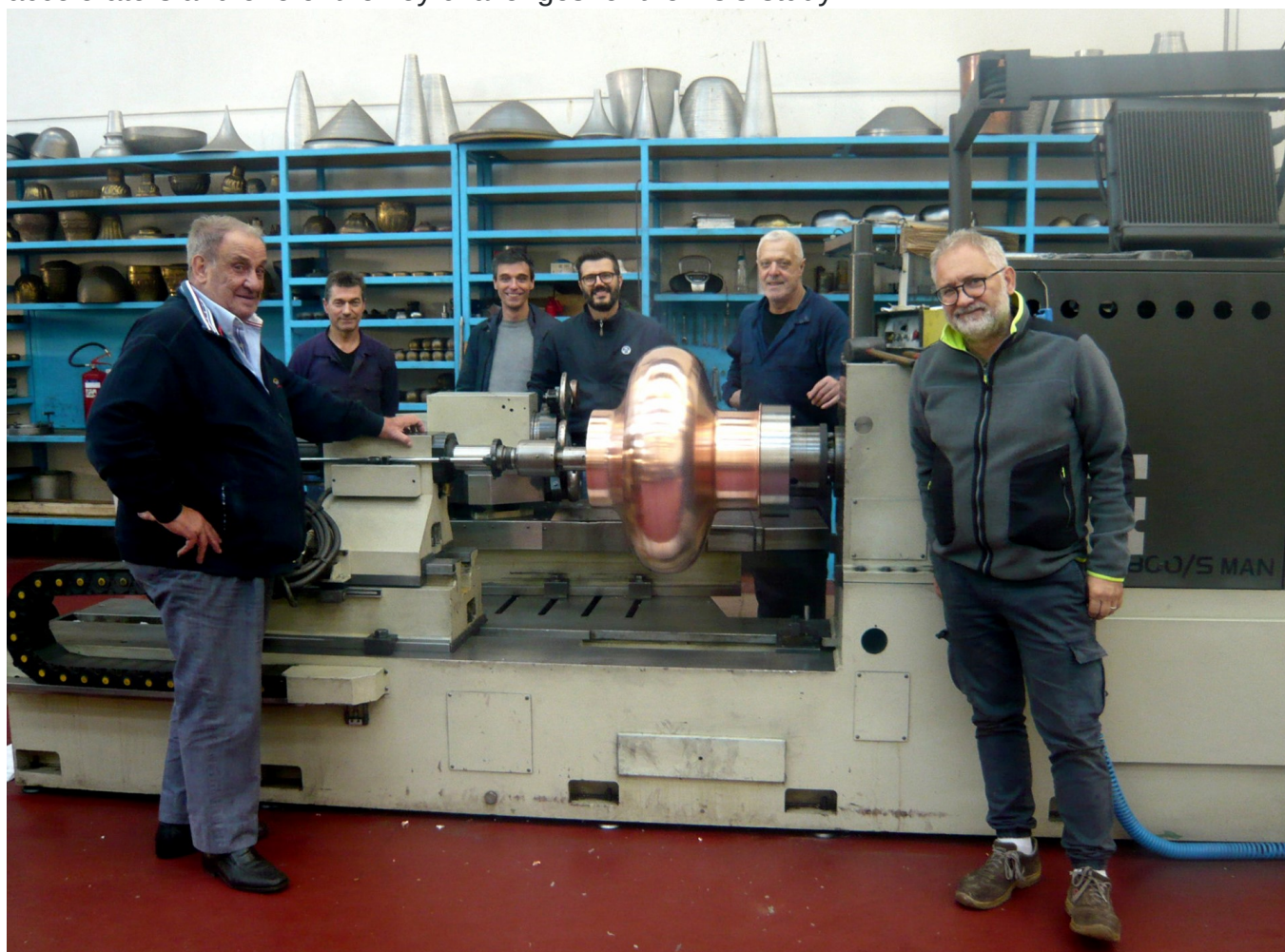
Header Image: The teamwork with the first copper seamless 400 MHz cavity. (Image: C. Pira)
