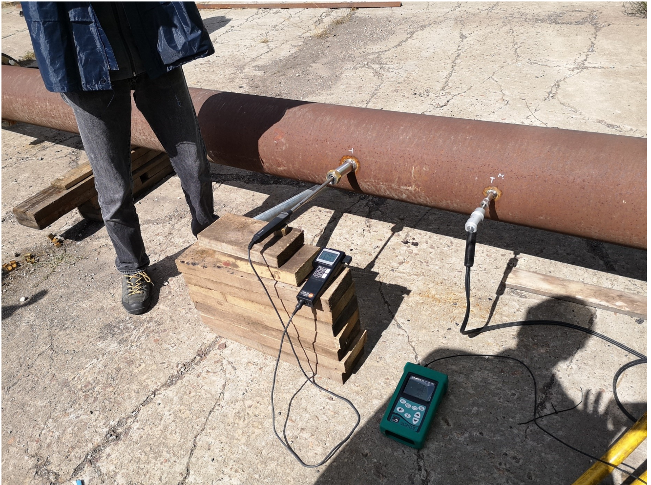
Measurement of exhaust composition. (Image: ARIES)
