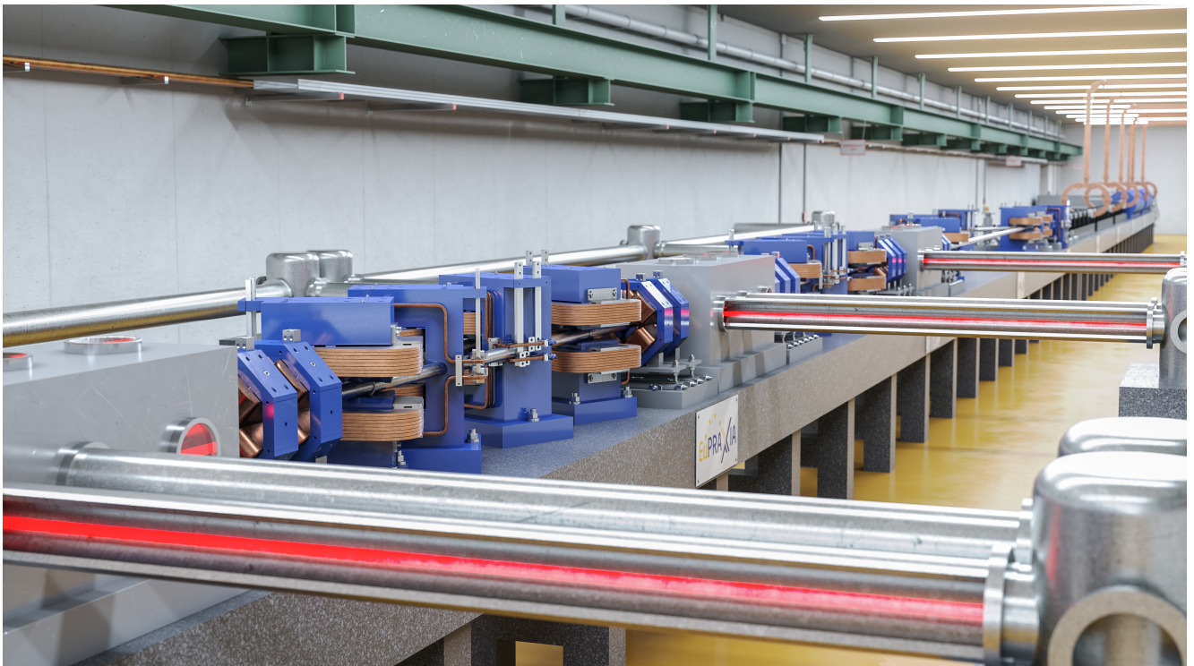
Rendering of the two-stage, very low energy spread plasma accelerator developed for the EuPRAXIA facility. The open tubes show the paths of the laser pulses (red lines) that drive the plasma wakefields in the vacuum chambers. (Image credit: EuPRAXIA)
