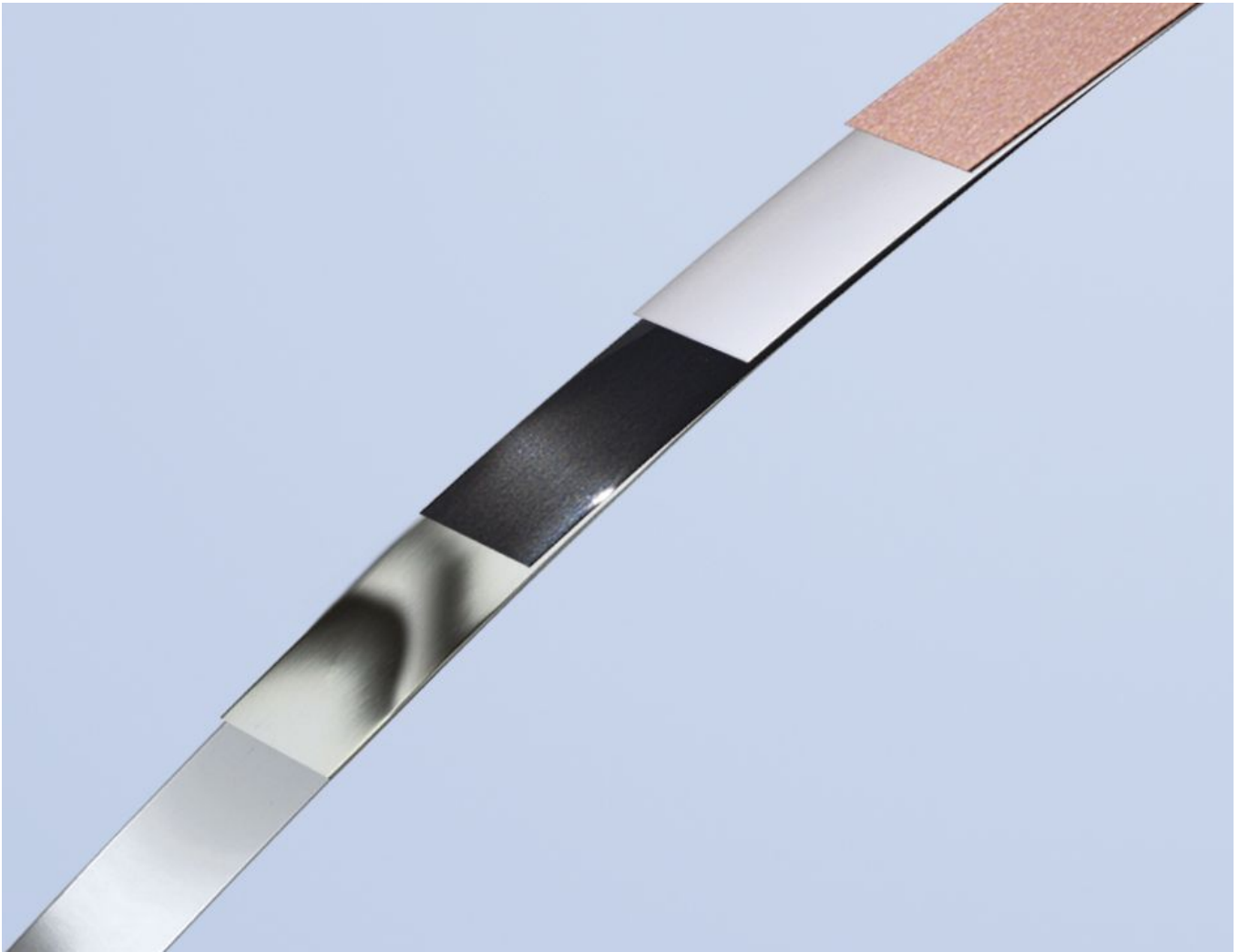
The 12 mm HTS tape manufactured by Bruker BHTS in the context of the H2020 ARIES project. (Image: Bruker/ARIES)
