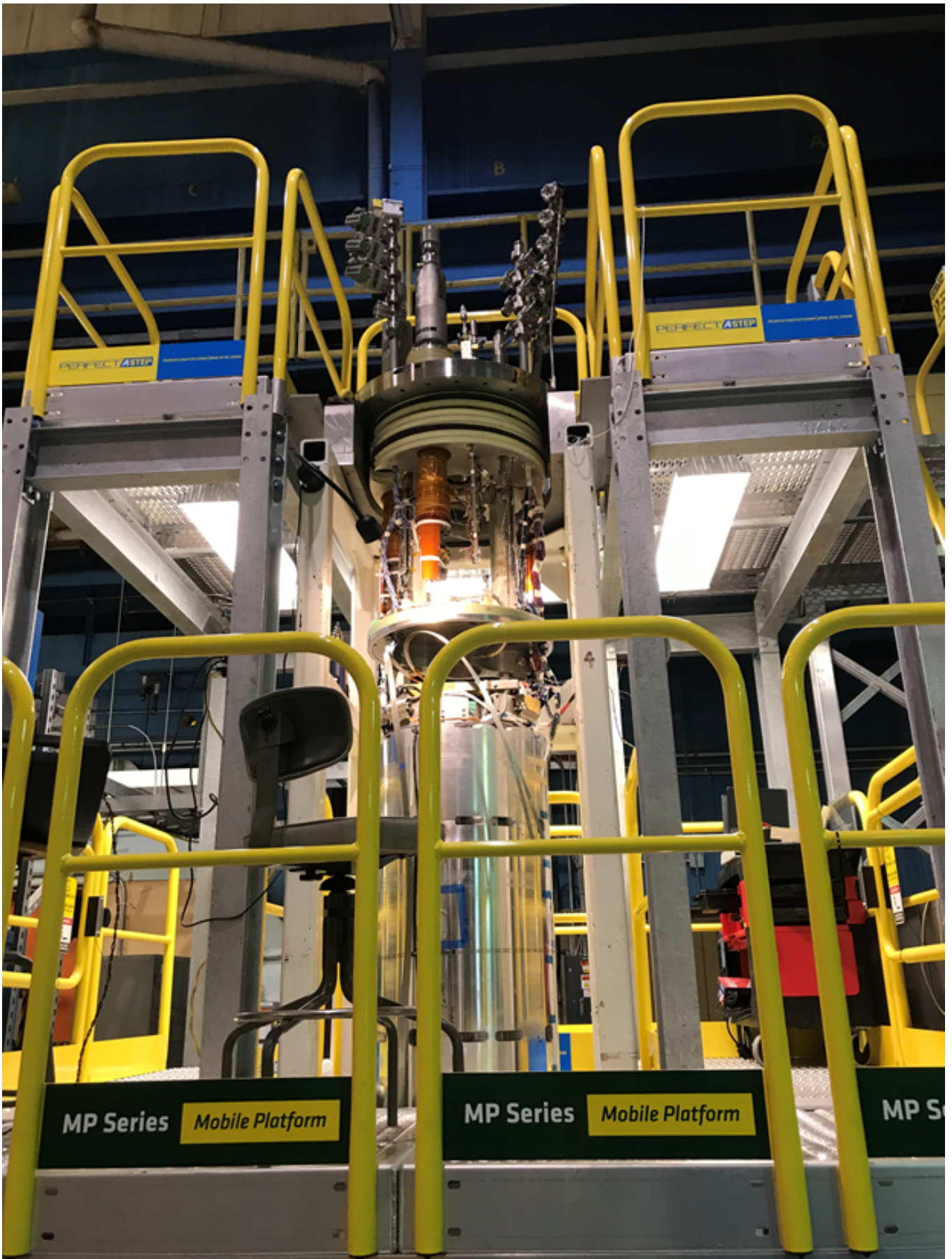
The quadrupole magnet being prepared for a test at Brookhaven National Laboratory. (Image: Brookhaven National Laboratory)
