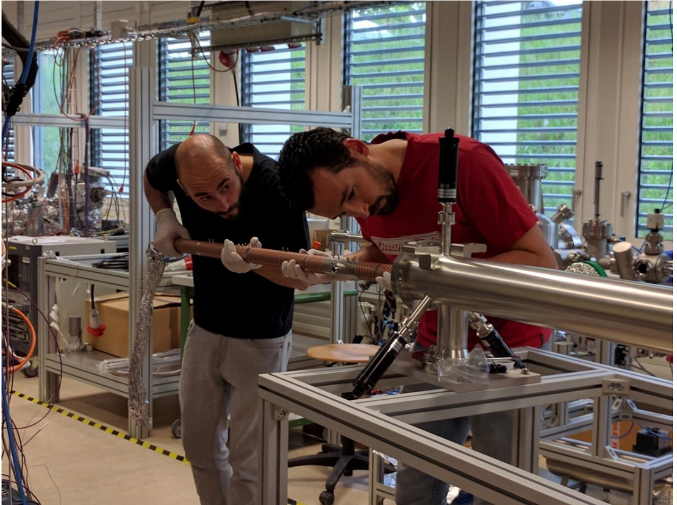
Fig.2: Left Luis Antonio González, Right Left Miguel Gil-Costa during installation of the first FCC-hh beam screen prototype for commissioning at BESTEX. (Image: FCC)
