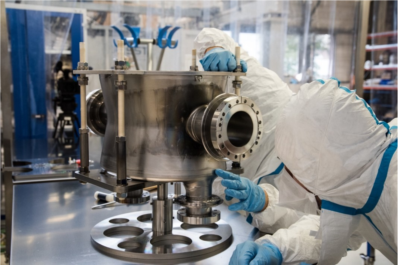
Figure 1: DQW Crab Cavity Prototype being assembled at CERN.
