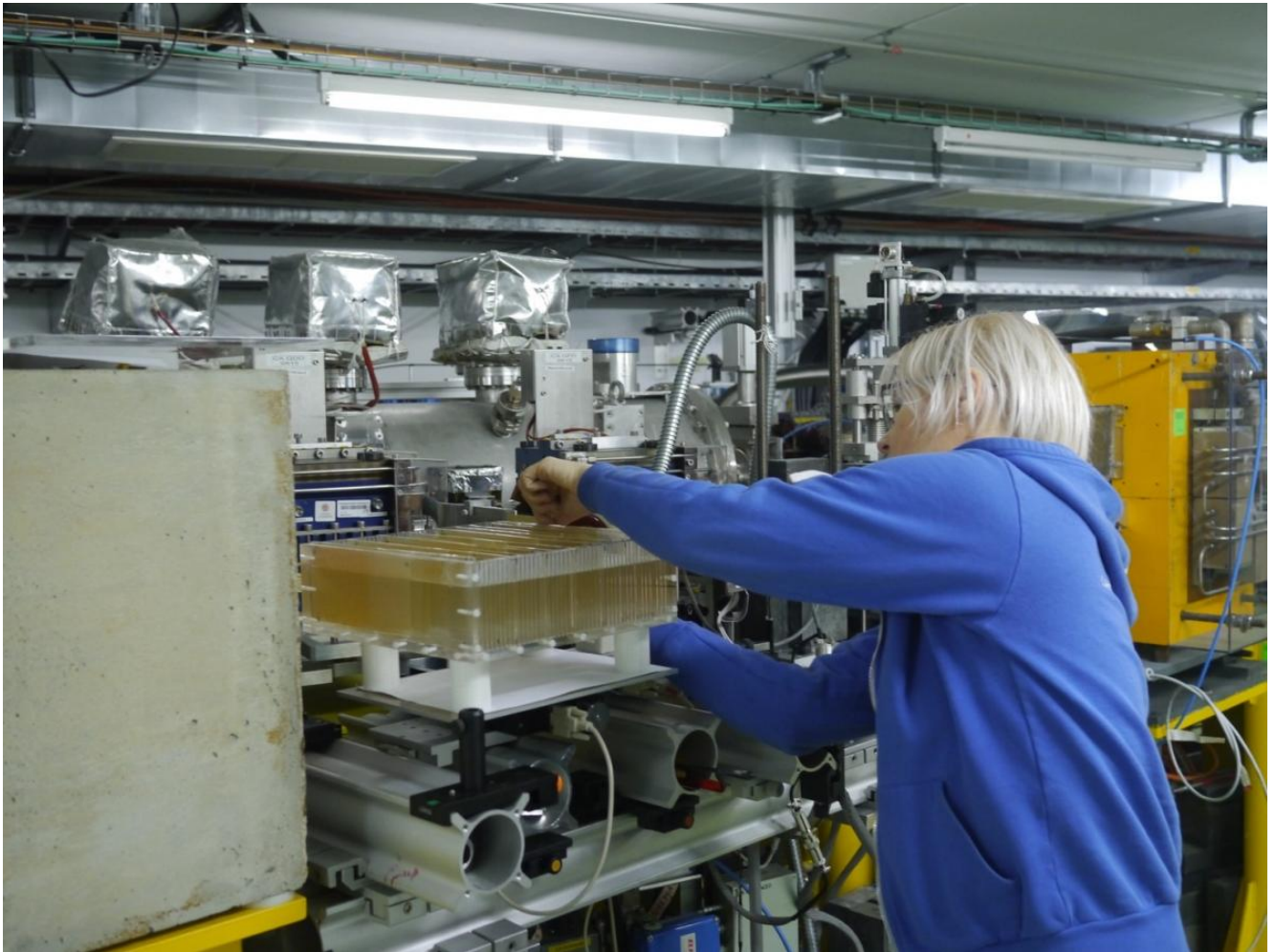
Water phantom being installed on the VESPER test stand by Agnese Lagzda – Manchester University. (Credit: Kyrre Ness Sjoebaek - kyrre.ness.sjoebaek@cern.ch)
