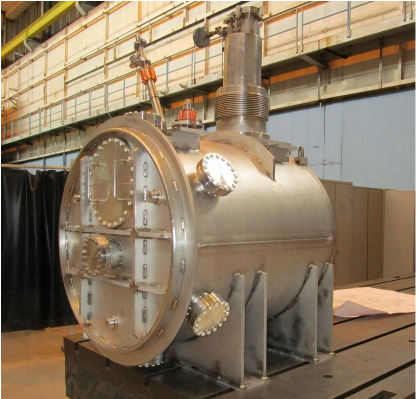
Fig.3: Cryostat housing CCC monitor. (Credit: CERN)
