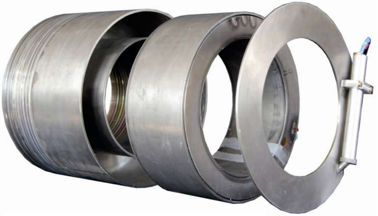
Fig. 5: CCC magnetic superconducting shield and ferromagnetic pickup coil. (Credit: University of Jena)
